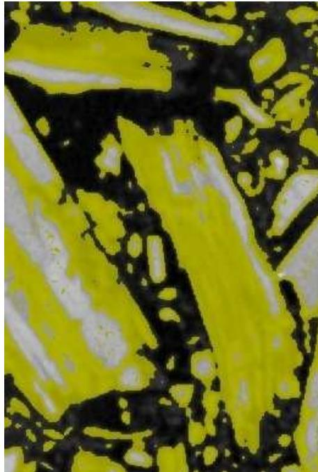
**Figure 5. 20:** Image of the wollastonite sample after 168 hours of carbonation process. The yellow parts indicate the presence of CaCO<sub>3</sub>. The gray covers presence of CaSiO<sub>3</sub> and SiO<sub>2</sub>.
